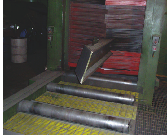
A member exits a rotary blast machine. Photo courtesy of Zimmerman Metals, Denver.
