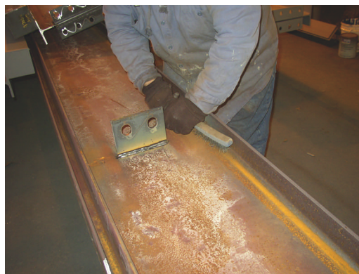
A worker uses a wire brush to prepare a member to SSPC-SP2. Photo courtesy of Atlas Iron Works, St. Louis.
