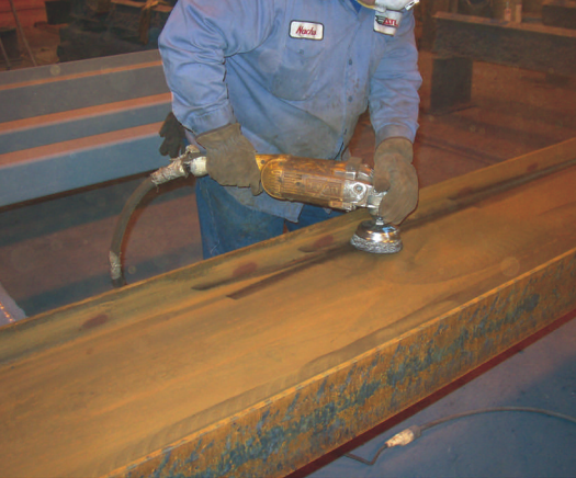
A worker prepares a member to category SSPC-SP3. Photo courtesy of Atlas Iron Works, St. Louis.
